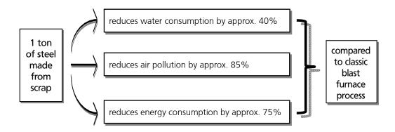
Electric steel mills play an important role in industrial society's materials cycle, because they produce steel from scrap metal. Charging materials for electric steel mills include scrap from vehicles (shredded scrap), demolition scrap and new scrap like sheets and turnings.
