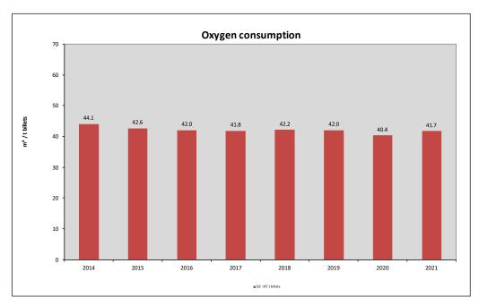
In 2021, oxygen consumption was slightly higher than in the previous year due to changed boundary conditions, a changed scrap mix and the resulting adjustment in operation mode.
