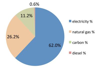
The energy carriers at BSW are electrical energy, natural gas, coal and diesel fuel. The percentage of renewable energies (according to EEG) from externally sourced electricity in 2021 was 1.8 % according to suppliers' statement. Carbon is mainly used for the generation of foaming slag but will also be considered.
