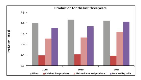
The difference between steel plant and rolling mill production results from production related losses in the rolling mill (internal scrap from the shears and scale). Furthermore, billets are processed into wire in other wire rod mills.
